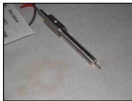
同軸型熱電対 (MEDTHERM)
