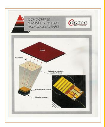
Measuring radiant flux with no intermediary temperature differences leads to cancel the thermal noise that is a fundamental limit to radiant measurements.
