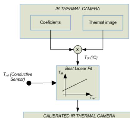
Fig. 6 In situ Thermal Camera calibration
