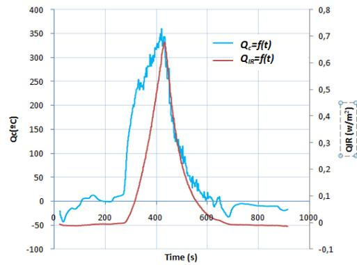
Fig. 9 Conductive heat flux VS Radiative heat flux
