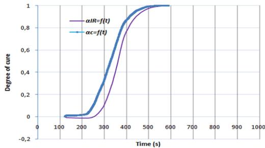
Fig. 11 Computed degree of cure measured by both sensors.
