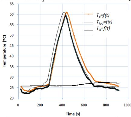
Fig. 7  $T_{log}$  is Reference Temperature (log) VS  $T_c$  temperature in the conductive sensor and,  $T_A$  is the ambient temperature.
