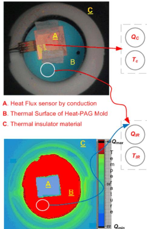
Fig. 4. Setup of the experiment. Thermal Photo in an instant time.
