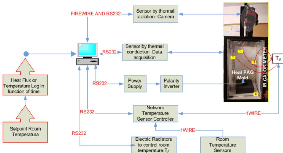
Fig. 5. Software and Hardware as integration tools for studying cure stage by Heat PAG Mold.
