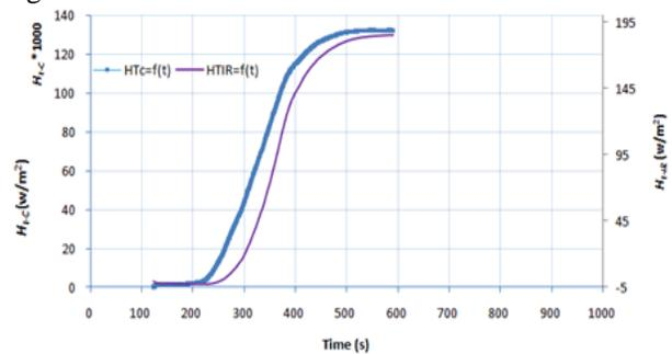
Fig. 10 Energy emitted measured by each sensor.
