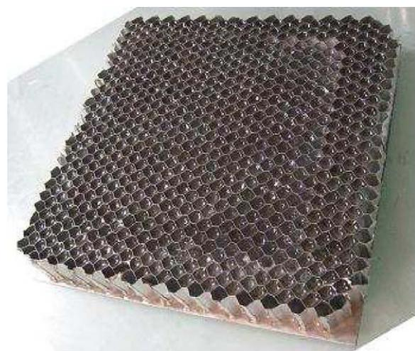
**Fig. 2.** Honeycomb panel sample filled with paraffin, before to stick the upper aluminium skin.
