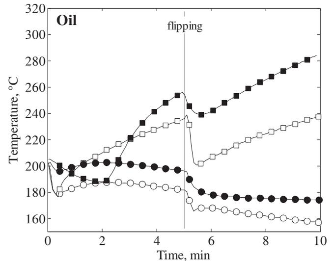
**Fig. 1.** Evolution of pan temperatures under a centrally-placed product during the pan-frying of three breaded poultry products on an electric hob without or with a thin layer of oil.
