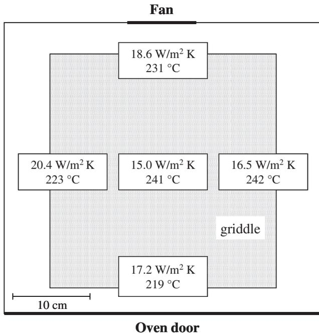
Fig. 4. Heat transfer coefficient ( $W/m^2 K$ ) and equivalent radiative temperature ( $^{\circ}C$ ) measured at different locations within the baking chamber during heating tests with oven #1 operating at  $240^{\circ}C$  under forced convection.
