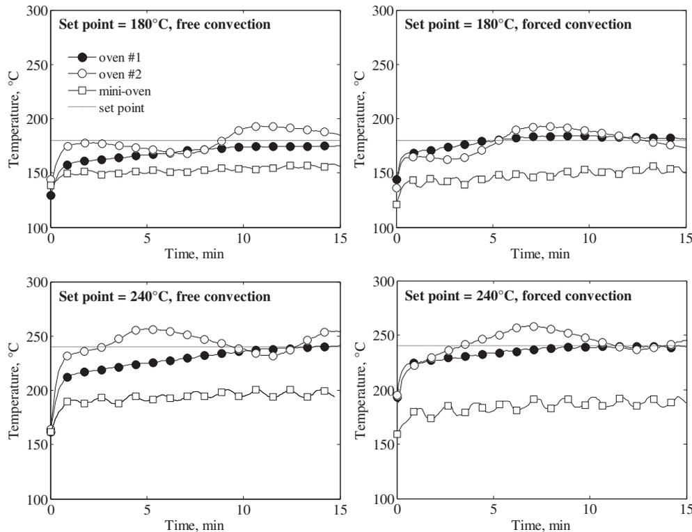
**Fig. 2.** Evolution of air temperatures during the oven-baking of three breaded poultry products under free or forced convection at a set point of  $180^{\circ}\text{C}$  or  $240^{\circ}\text{C}$ .
