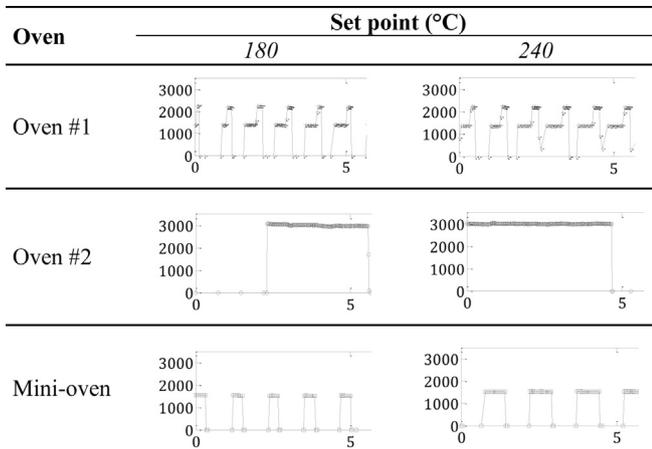
**Fig. 3.** Current power profile under forced convection during the first minutes of heating products in an oven. Time (min) on the x-axis and current power (W) on the y-axis.
