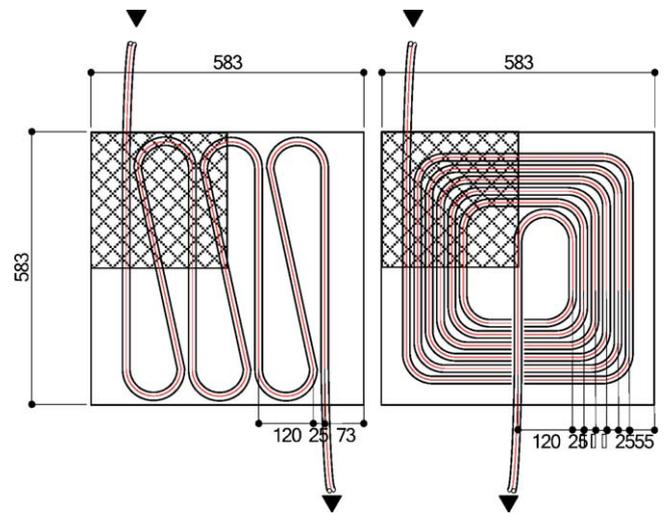
Fig. 2. Detail of panels used in the experiment: (left) meandering type and (right) spiral type. (Cross-hatched area is heat flow sensor)
