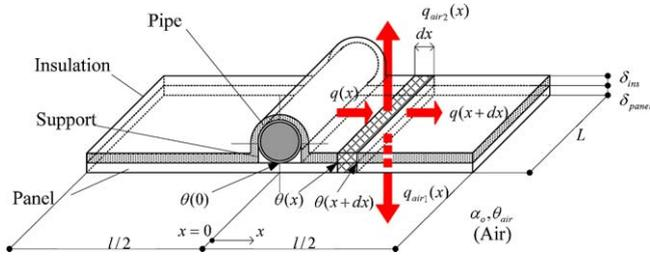
Fig. 7. Model for a panel bonded with piping.
