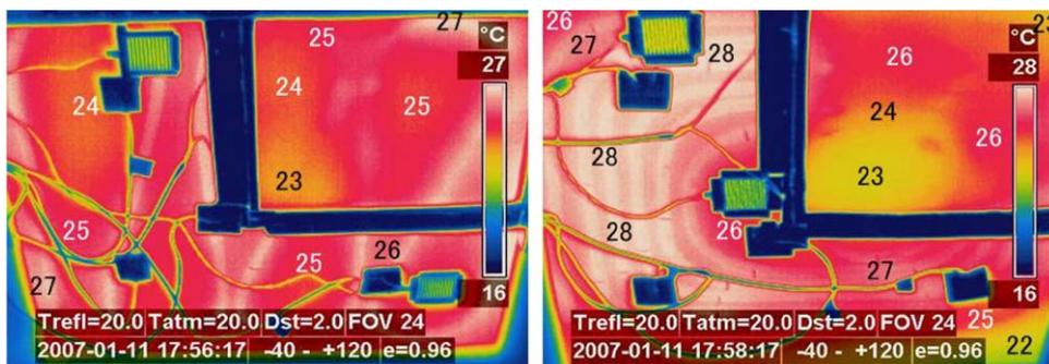
Fig. 6. Thermal images for Case 12 (left) meandering and (right) spiral (heating, room temperature 18 °C, supply water temperature 33 °C).
