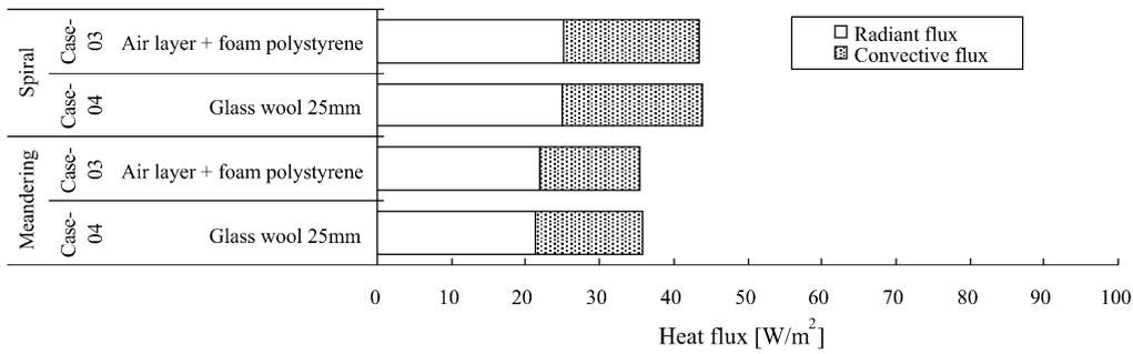
Fig. 3. Breakdown of heat flux for Case 03–04 (cooling, room temperature 28 °C, supply water temperature 18 °C).
