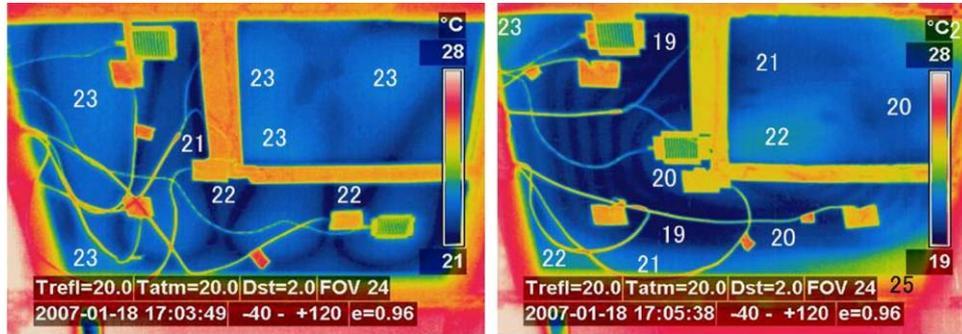
Fig. 4. Thermal images for Case 03 (left) meandering and (right) spiral (cooling, room temperature 28 °C, supply water temperature 18 °C).
