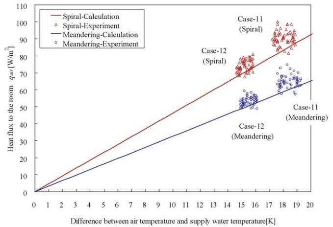
Fig. 8. Comparison between calculation and experiment data: (above) cooling and (below) heating.
