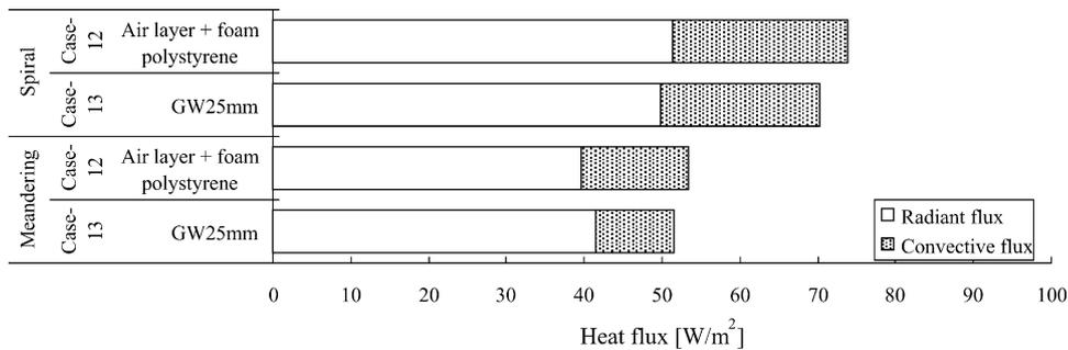
Fig. 5. Breakdown of heat flux for Case 12–13 (heating, room temperature 18 °C, supply water temperature 33 °C).
