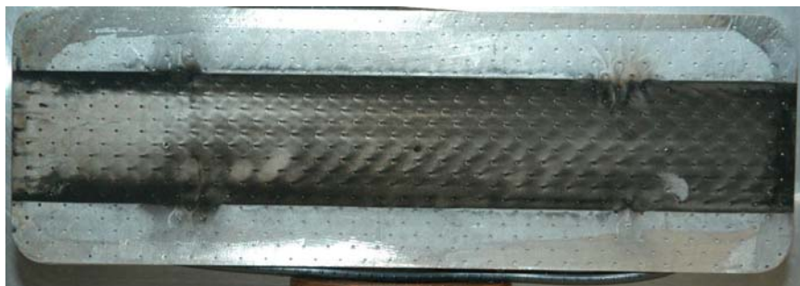
Figure 15. Soot patterns were helpful for making a qualitative assessment of cooling performance.
