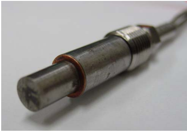
Figure 5: Fast-response coaxial heat flux probe with surface junction shown
