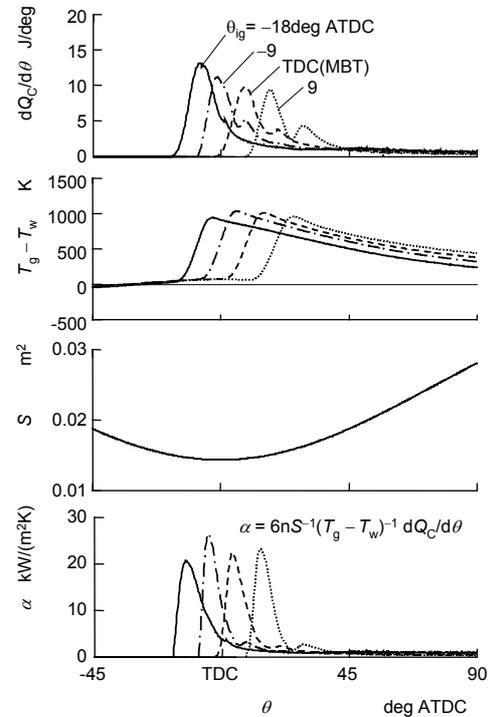
Fig.3 Rate of cooling and heat transfer coefficient derived from experiment by heat release analysis
