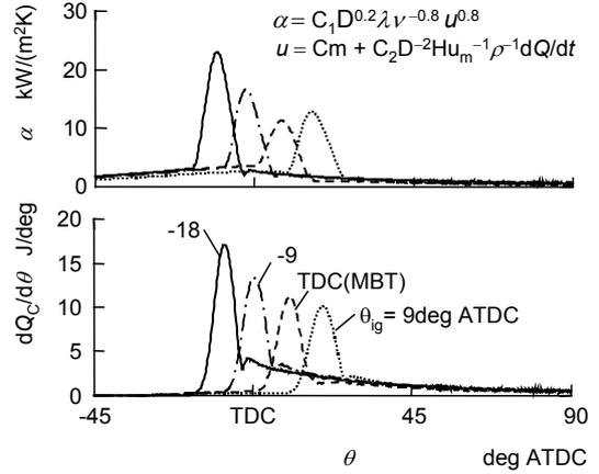
Fig.8 Heat transfer coefficient and rate of cooling calculated by turbulent heat transfer equation with the new velocity term
