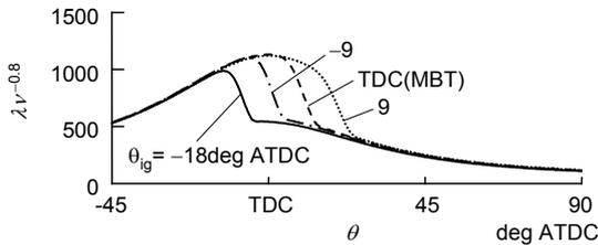
Fig.4  $\lambda \nu^{-0.8}$  of in-cylinder gas during combustion
