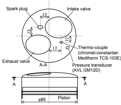
Fig.2 Combustion chamber of the tested engine
