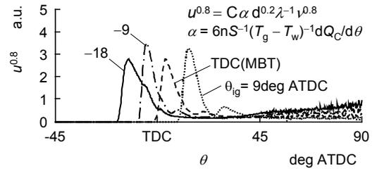
Fig.6 Representative velocity of in-cylinder gas derived from experiment
