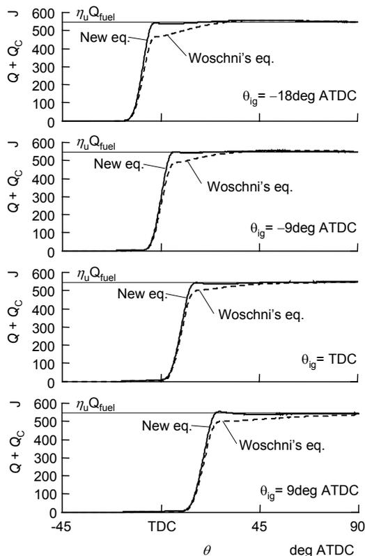
Fig.10 Cumulative real heat release calculated by the new heat transfer equation for different ignition timings
