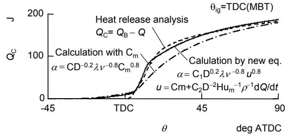
Fig.9 Cumulative cooling loss calculated by the new heat transfer equation
