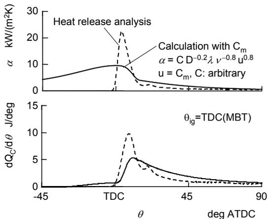
Fig.5 Heat transfer coefficient and rate of cooling calculated by turbulent heat transfer equation with mean piston speed
