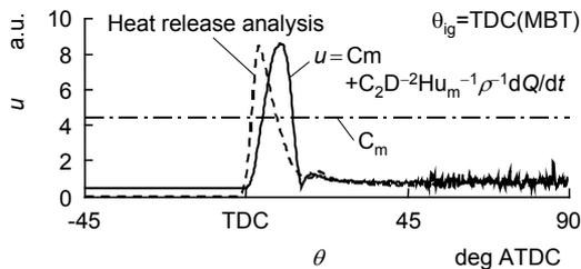
Fig.7 New velocity term employing heat release rate
