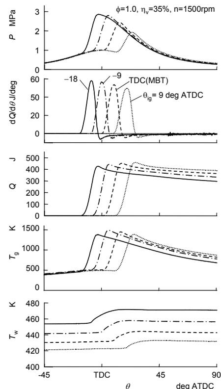
Fig.1 Stoichiometric combustion of hydrogen with different ignition timings
