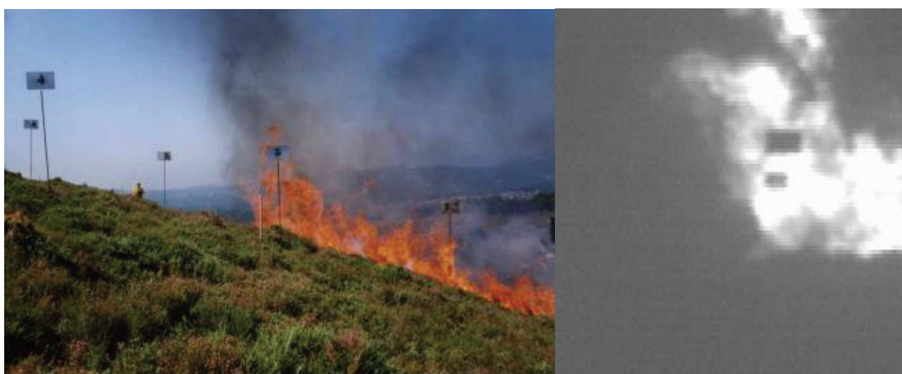
Figure 3-11: Fire progression during Galician experiments registered using a visual (left image) and an infrared (right image) camera.
