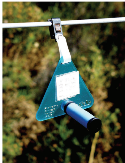
Figure 3-17: Photograph of a passive sampler used in Gestosa fire experiments.
