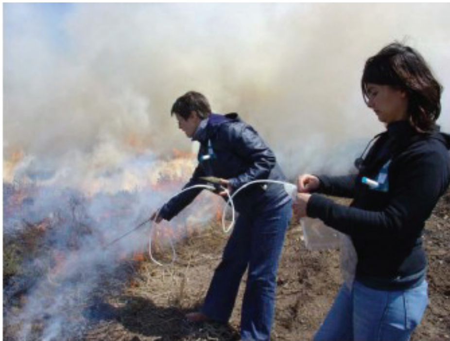
Figure 3-15: Smoke sampling technique during smouldering phase.
