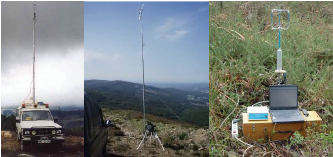
Figure 3-7: Meteorological mast (10 m height), mobile automatic meteorological station and ultrasonic anemometer.
