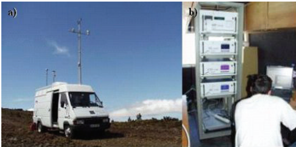
Figure 3-16: Mobile laboratory used by UAVR team during Gestosa experiments for air quality and meteorological data acquisition.
