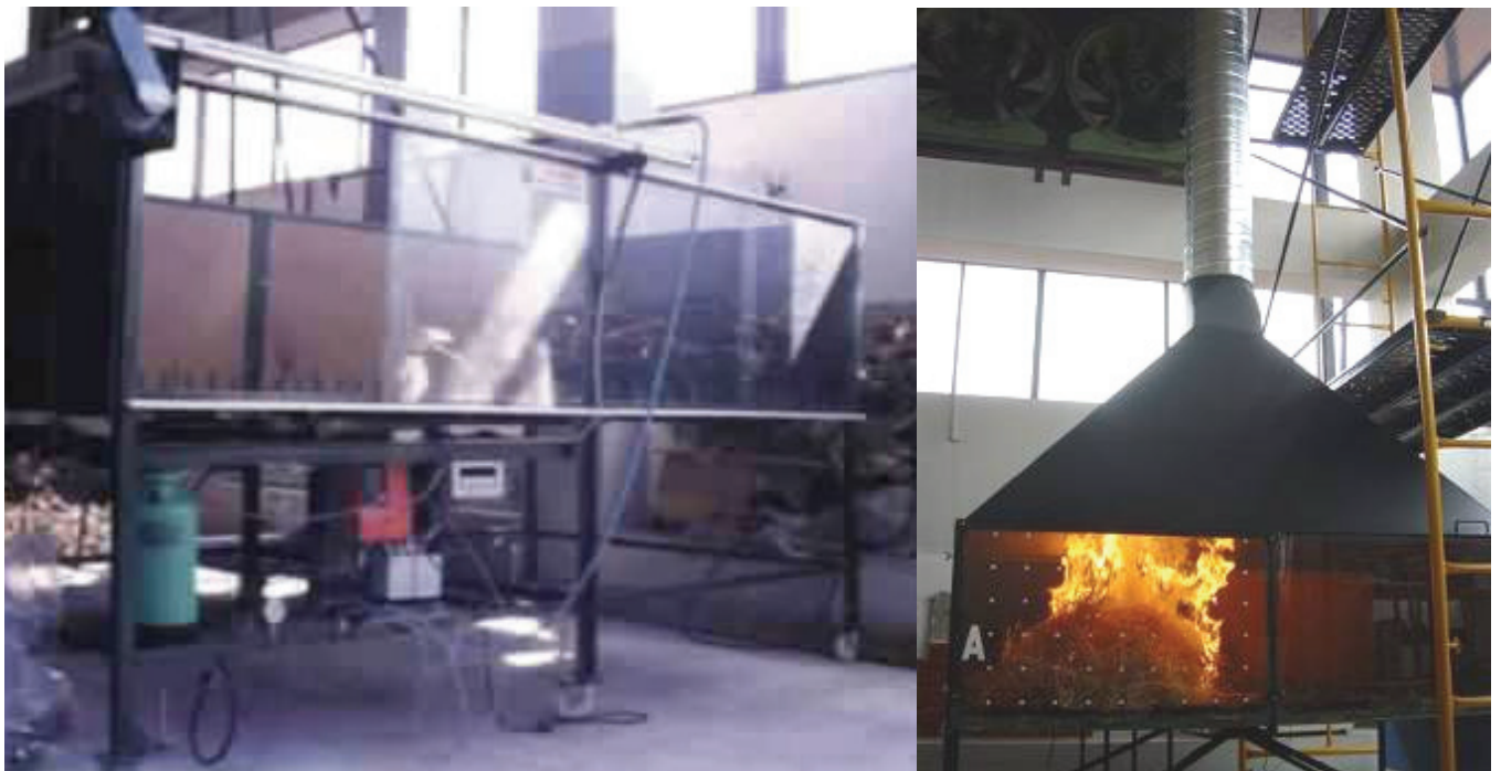
Figure 2-2: Combustion table before (on the left) and after (on the right) the adaptation to emissions measurement.
