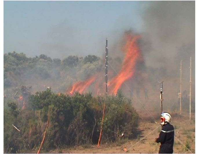
Fig. 11. Flame tilted by the wind.
