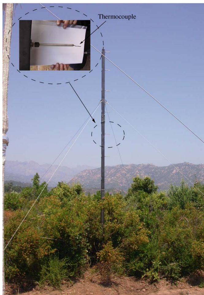
Fig. 7. Measuring structure for gas temperature: mast and set-up for the thermocouple protection.
