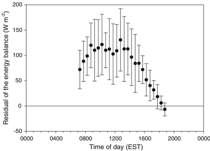
**Fig. 3** Mean energy balance residual at site 13 as a function of the time of day including the standard deviation for the entire observation period from 27 June to 6 August 2008. A positive residual implies that the available energy is larger than the sum of the turbulent fluxes
