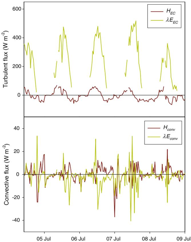
**Fig. 4** Turbulent energy fluxes at site 13 as measured by the temporal eddy-covariance method (*top panel*) and convective fluxes (*bottom panel*) for the period from 4 July to 9 July 2008
