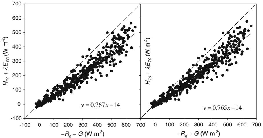
**Fig. 2** Energy balance scatter plots with linear regression for the pure turbulent fluxes (*left panel*) with 30-min averaging time and the atmospheric fluxes including the convective contribution (*right panel*); all terms positive for fluxes away from the surface
