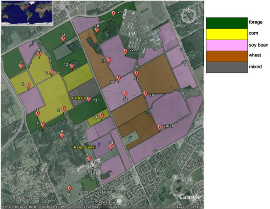
**Fig. 1** Overview of the measurement set-up with land use information. The locations of the 25 HOBO temperature/humidity sensors are indicated by red pins labelled with a T and the site number. This image covers an area of approximately 5 km by 5 km
