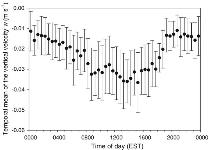
**Fig. 5** Temporal mean of the vertical wind velocity at site 13 as a function of the time of day including the standard deviation for the entire observation period from 27 June to 6 August 2008
