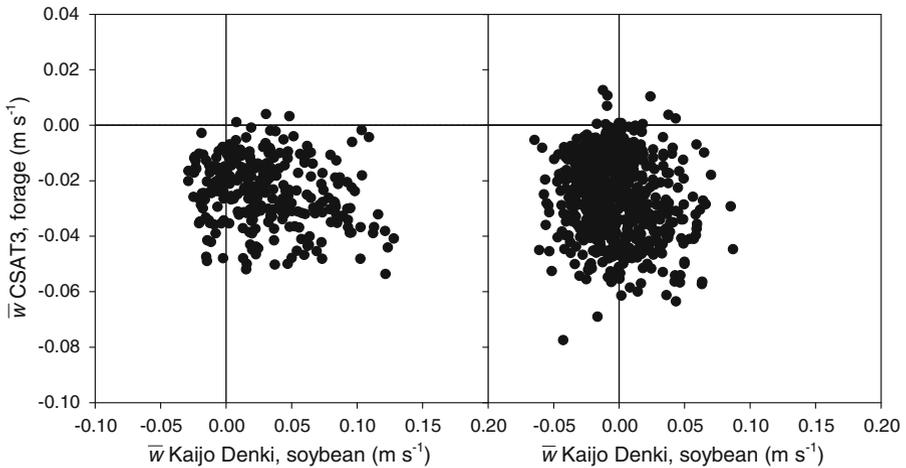
**Fig. 9** Vertical wind velocities  $\bar{w}$  at the central site measured over grass (CSAT3) versus  $\bar{w}$  over bare soil/soybean (Kaijo Denki) for the period before (*left*) and after (*right*) 7 July 2008, when the soybean crop reached a height of 0.15 m
