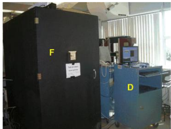
Fig 3 On the Left, location of (H) mould for square part to be manufactured on the (G) table which is sensed by means of (A) thermal camera, (B) visible camera, (C) contact Heat Flux-Temperature sensors and (E) surroundings temperatures sensor. Moreover, (F) is mean, black box is opened. On the Right, (F) is closed which is made of wood for the thermal-protection to experimentation that avoids convection, sudden thermal disturbs into the tests, and finally, (D) is the acquisition system by computer.
