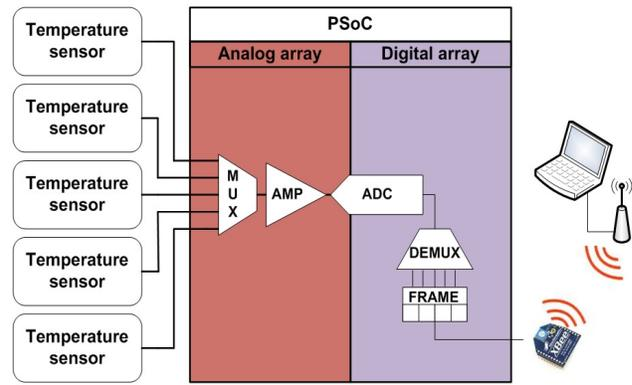
Figure 2: acquisition system architecture based on a PSoC™ programmable component.
