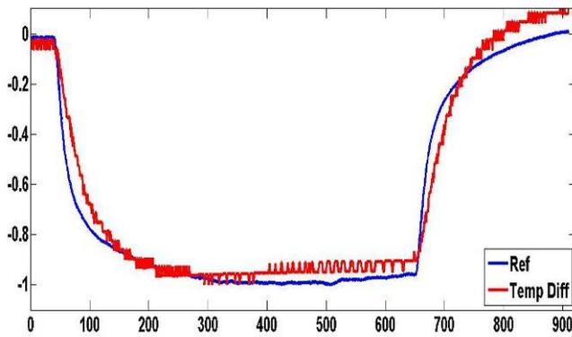
Figure 3: comparison of the two normalized heat flux, the reference in blue and the calculated heat flux (by temperature difference) in red.
