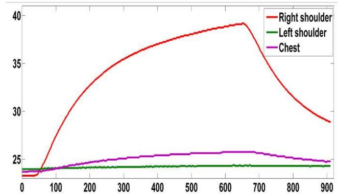
Figure 4: temperature recording in the outer garment on right (red) and left (green) shoulders and in the chest area (purple) in °C.
