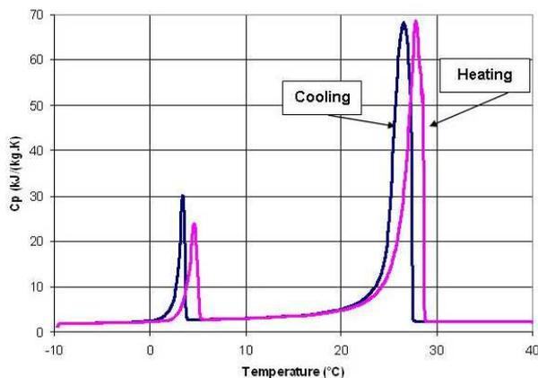
Figure 1. Stored heat ( $\sim C_p$ ) as a function of temperature measured by Differential Scanning Calorimetry (Scanning rate, 0.05 K/min)
