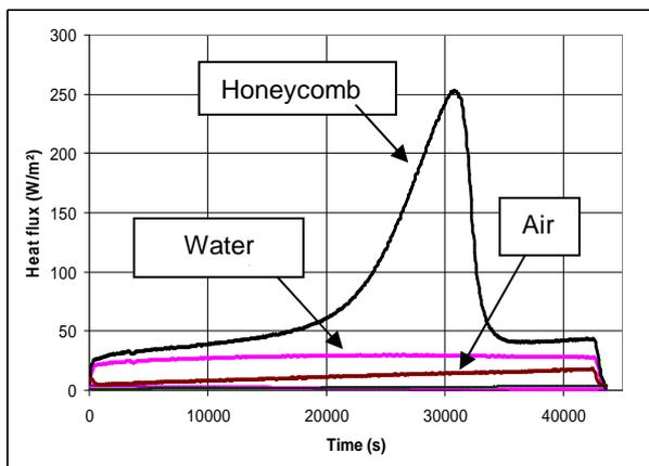
Figure 7. Heat fluxes measured at the front sides of the three samples (PCM, water, air) during sample heating. Fluxes measured at the back sides are nearly zero.
