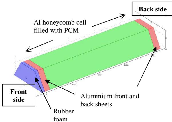
Figure 9. Structure for the finite element modelling. Half of an aluminium hexagonal cell filled with PCM is represented with aluminium sheets of both sides. Rubber foam is placed on the front side.
