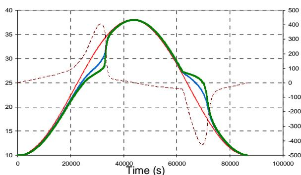
Figure 11. Numerical prediction for temperature (full lines) and flux (dotted line) variations of the PCM-filled honeycomb sample.
