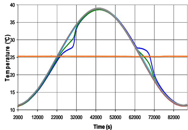
Figure 8. Temperature variation for sinusoidal cycle. Pure sine curves are for imposed temperature, and front side temperatures of water and air samples.
