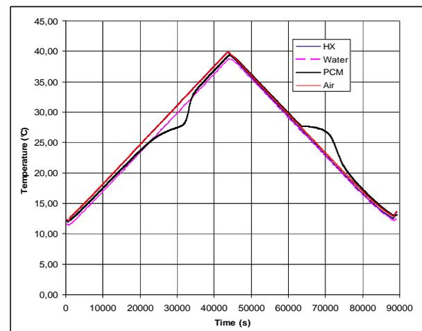
Figure 5. Temperature variations on the back side of the empty sample (Air), the sample filled with water (Water) and the honeycomb sample filled with PCM (PCM). Temperature of the heat exchanger (HX) is given for comparison.
