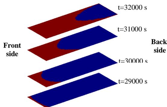
Figure 10. Melting front propagation within the PCM in the symmetry plane of a honeycomb, for the time range [29000:32000].
