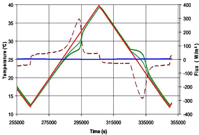
Figure 6. Temperature (full lines) and flux (dotted line) variations of the PCM-filled honeycomb sample.
