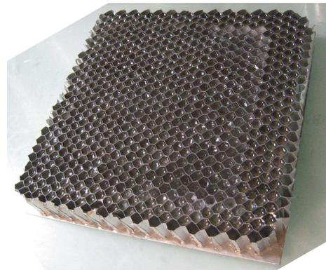
Figure 2. Honeycomb panel sample filled with paraffin, before to stick the upper aluminium skin.
