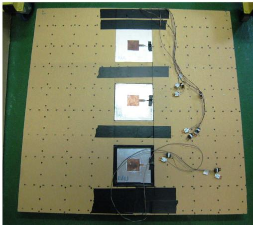
Figure 4. The panel placed in the test loop. Three samples from up to down: Empty (Air), filled with PCM, filled with water.
