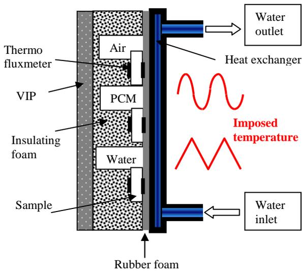
Figure 3. Schematic of the test section with three samples and with temperature and flux sensors
