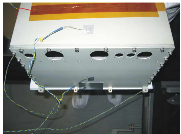
Figure 11 – Sensor layout. In the figure it is possible to see sensor n° 8 placed near the heater and sensor n° 10 placed on a lateral wall.
