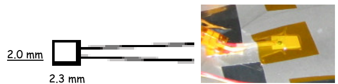
Figure 6 - PT100 temperature sensor used to monitor and control the temperature of the equipment under test.
