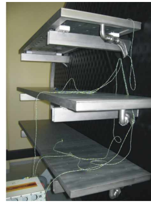
Figure 9 – The shroud and cold plates of the space simulator.
