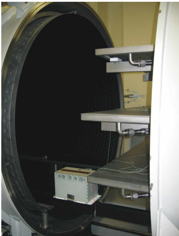
Figure 13 – The test item placement inside the Thermo-vacuum chamber.
