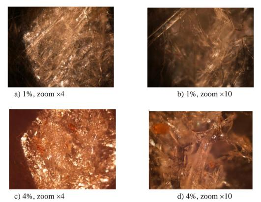
The optical microscopy enabled assessment of the microstructure of the biofoam which was composed of entangled filaments or leaves. The 1% biofoam appeared to be less compact than the 4% biofoam which may have been due to a dominating filament-based microstructure. In order to investigate this point in more detail, the SEM results are presented in Figure 2.
