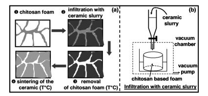
In step 3, the filled foam was dried and slowly centrifuged to eliminate the excess impregnated slurry. Then, the polymer part was removed by thermal treatment. The final step concerned the sintering of the ceramic material exhibiting open porosity rate whose shape was close to that of the solid skeleton of the initially infiltrated chitosan foam.
