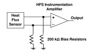
Figure 4 - Simplified Heat Flux Signal Circuit Diagram
