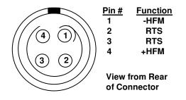
Figure 3 - Female Lemo Connector Pin Out
