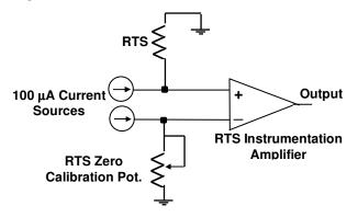
Figure 5 - Simplified RTS Signal Circuit Diagram
