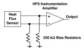
The TC char**Figures**4sv**Sichpithed**4**Heag**4**hs**x**SignalOCir2OIt DOOgrand** 1000. The circuit configuration is otherwise just like the HFS channel, i.e. with two bias resistors (200 k $\Omega$ ) placed from the inputs of the amplifier to ground, etc. The TC signal may be set to zero at any desired temperature between 0°C and 250°C. See Temperature Measurements Using the Thermocouple.
