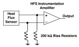
Figure 4 - Simplified Heat Flux Signal Circuit Diagram
